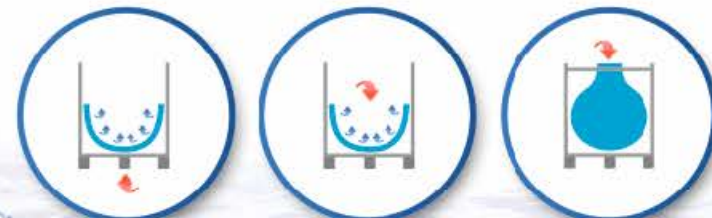
filling through the bottom valve filling through the top valve filling using a filling bridge
